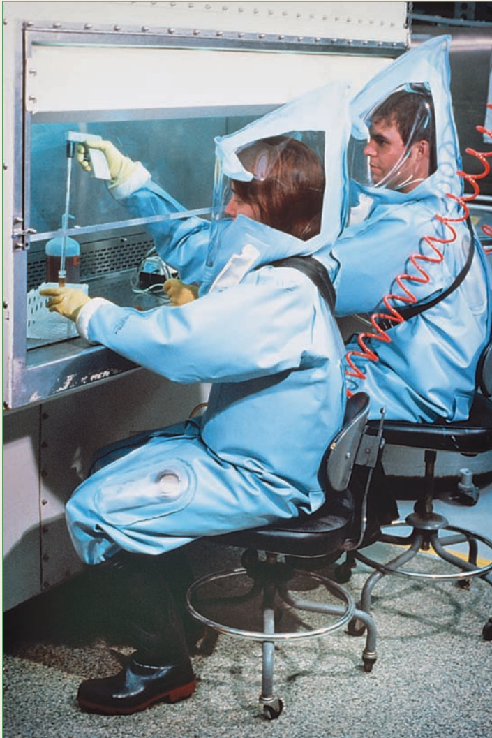
Figure 3.2 Workers in a biosafety level 4 (BSL-4) laboratory must carry out their work dressed in “space suits,” and undergo extensive decontamination prior to returning to pathogen-free areas. Those who work in these labs do research on the most deadly agents known to mankind.
